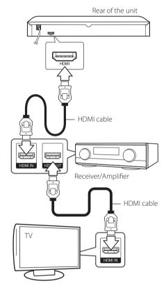
Connect the amplifier's HDMI output jack to HDMI input jack on your TV using an HDMI cable if your amplifier has HDMI output jack. (Refer to amplifier's owner's manual)
