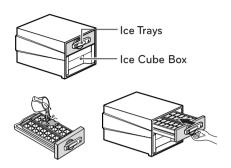
• To remove ice cubes, hold the lever of the tray and pull turn gently. Then, ice cubes drop in to the ice cube box.
