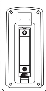
Remove the battery cover on the rear of the Remote Control, and insert one (size AAA) battery with **+** and **-** matched correctly.
