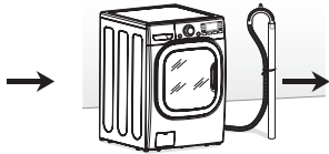
Connecting the drain line
