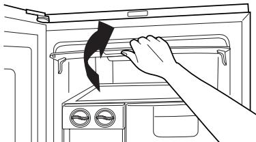
1. Grip the handle of flap cover, then rotate and lift.
