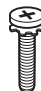
Stativskruvar 8EA, M4 x L20 (Endast UB85**-ZA, UB93**, UB95**-ZA) 4EA, M4 x L20 (Endast UB85**-ZD, UB95**-ZB, UC97**) (Se sid. A-3, A-4, A-8)
