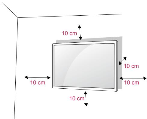
If you intend to mount the monitor to a wall, attach a Wall mounting interface (optional parts) to the back of the set.
