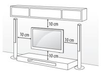
Make sure to use screws and wall mount bracket that meet the VFSA standard. Standard dimensions for the wall mount kits are described in the following table.
