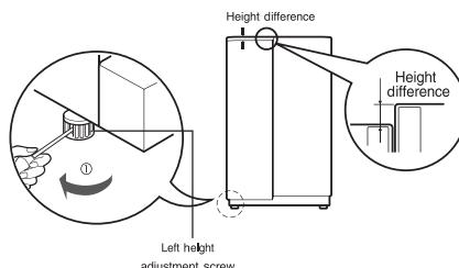
**If the freezer compartment door is higher than the refrigerator compartment door**
