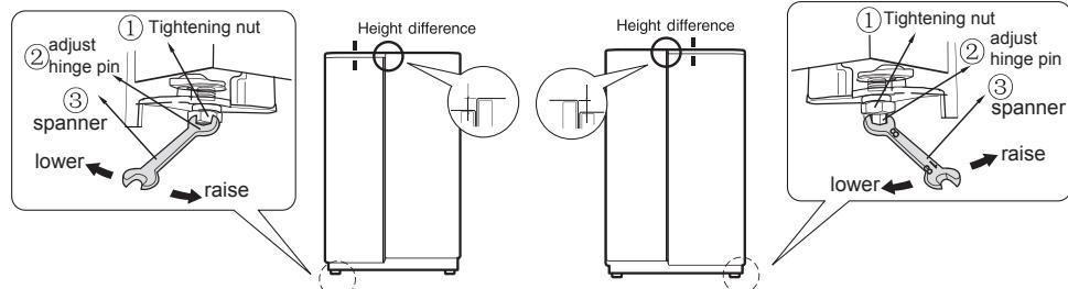
Do not adjust the height excessively. You can lose the hinge pin.
