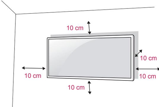
To install the monitor to a wall, attach a wall mounting bracket (optional) to the back of the monitor. Make sure that the wall mounting bracket is securely fixed to the monitor and to the wall.
