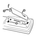
Remove the battery cover on the rear of the Remote Control, and insert one (size AAA) battery with
