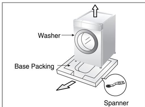
1. Remove the cardboard box and styrofoam packing.
