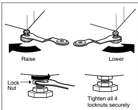
2. If the floor is uneven, turn the adjustable feet as required. (do not insert pieces of wood etc. under the feet)
