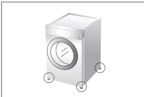
1. Leveling the washing machine properly prevents excessive noise and vibration. Install the appliance on a solid and level floor surface, preferably in a corner of the room.
