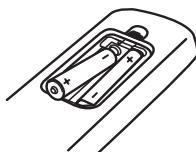
Remove the battery cover on the rear of the Remote Control, and insert two (size AAA) batteries with **+** and **-** matched correctly.
