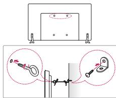
1 Insert and tighten the eye-bolts, or TV brackets and bolts on the back of the TV.
