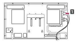
2 Mount the speaker by using a screw as shown in the following. Then connect the speaker cable.
