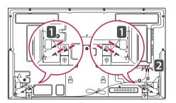
3 After installing your speakers, use holders and cable ties to organize the speaker cables.
