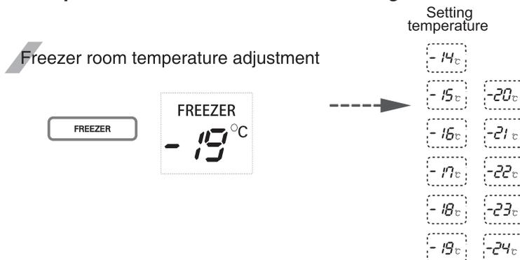
※ Whenever pressing **FREEZER** button, setting is repeated in the order of (-19°C → -20°C → ... → -24°C → -14°C → ... → -19°C).
