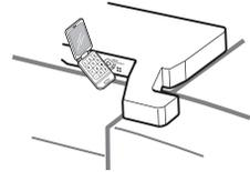
3. Hold the mouthpiece of your phone in front of the speaker that is located on the right hinge of the refrigerator door, when instructed to do so by the call center.
