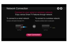
4 The device automatically tries to connect to the network available(wired network first).
