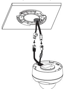
5. Assemble the camera and mounting bracket after align the front part of the camera and mounting bracket. Connect the unit by following step 1 and 2.
