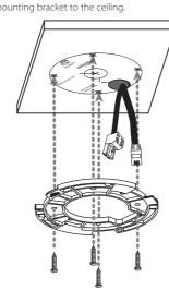
4. Connect the cables to the cable jacks of the camera body.
