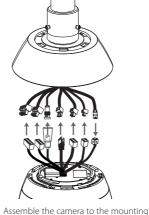
adaptor by turning it clockwise. Tighten the M3 SAMS Screws and then align the cover adaptor and main bod
