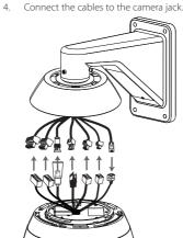
Assemble the camera to the mounting adaptor by turning it clockwise. Tighten the M3 SAMS Screws and then align the
