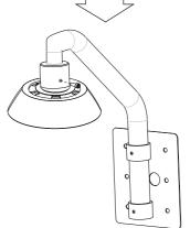
2. Drill a hole on the wall where you want to install the parapet. Pass the connection cable through the parapet mount assembly so that they hang
