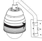
Assemble the camera to the mounting
