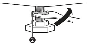
**4** Check if all lock nuts at the bottom of the appliance are secured properly.
