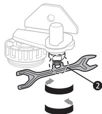
3 Fasten the keeper nut by turning it counterclockwise.
