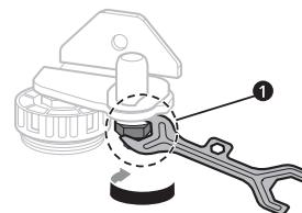
2 Turn the adjustment hinge pin clockwise or counterclockwise using the spanner ②. To lower the door, turn the adjustment hinge pin clockwise. To raise the door, turn the adjustment hinge pin counterclockwise.
