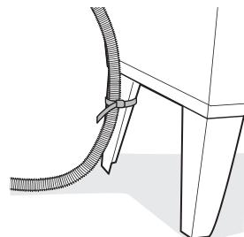
**4** If the water valves and drain are built into the wall, fasten the drain hose to one of the water hoses with the provided tie strap (3) (ribbed side on inside).
