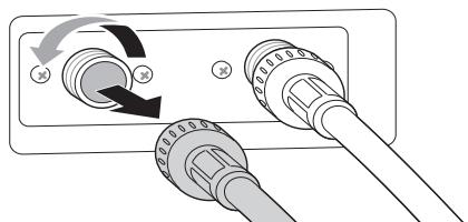
**4** Plug the power cord into a properly grounded electrical outlet.
