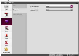
You can view all the channels in sequence in the selected screen division mode. You cannot use sequence mode with the 16 split (LRD5080 series: 8 split). While the sequence mode condition, if you change the screen division mode, the sequence function will be canceled.
