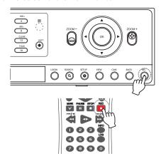
2. Press the REC button and then press the channel button you want to stop recording. If you stop instant recording, the recording mode will be changed into the scheduled recording mode (Continuous/ Sensor / Motion records). If the schedule is not set, the button indicator turns off and the recording type indicator turns gray on the selected channel screen of the main monitor.
