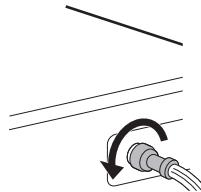
**2** Remove the water inlet filter with small pliers and then clean the filter using a medium bristle tooth brush.
