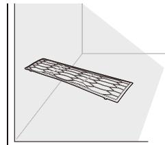
6 Insert the tabs on the air filter into the slots on the back of the front panel.
