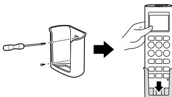
3 Slide the remote controller inside the holder.
