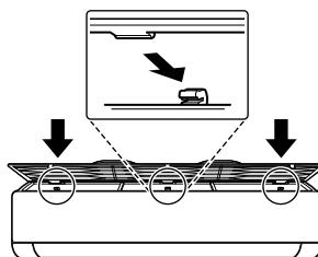
8 To make sure the filter is assembled properly, press down along the entire front length of the filter.
