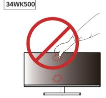
If you use the monitor panel without the stand base, its joystick button may cause the monitor to become unstable and fall, resulting in damage to the monitor or human injury. In addition, this may cause the joystick button to malfunction.
