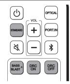
**STANDARD/BASS BLAST+**: Selects the sound effect. **DRC ON/OFF**: Makes comfortable sound at Dolby Digital.
