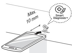
3 Press and hold the **Temp.** button for three seconds, while holding the phone mouthpiece to the icon or **Power** button.
