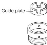
3 Push the adapter onto the end of the tap so that the rubber seal forms a watertight connection. Tighten the four fixing screws and the adapter ring plate.
