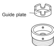
3 Push the adapter onto the end of the tap so that the rubber seal forms a watertight connection. Tighten the four fixing screws.
