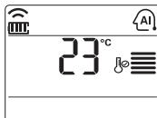
You can set desired temperature and indoor fan speed.
