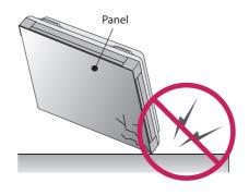
If the product is tilted onto the edge of the panel, the panel may be damaged.
