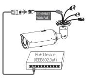
If the camera doesn't work properly after connecting PoE device, please check if the PoE device supplies enough power.
