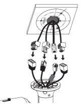
Follow the instructions below to ceiling or wall mount 3. Install the camera by using M4 Tapping screws to fix it on the ceiling.
