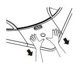
2 Open the PM1.0 sensor case on the side of the PM1.0 Sensor case and remove the rubber cap.
