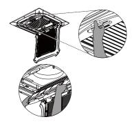
Remove the photocatalyst Deodorization filter by pulling upward.
