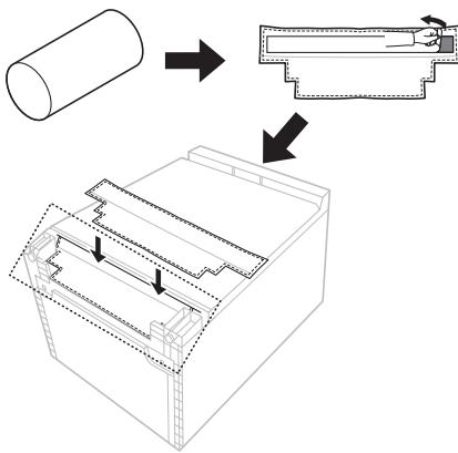
4 Remove the double-sided tape from the lower and front strips.
