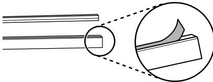
4 Attach the black coloured lower strip ① to the bottom of the lower cover.
