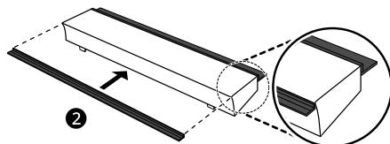
6 Attach the lower cover with the strip onto the appliance.
