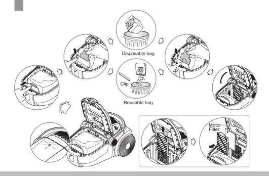
The dust bag needs changing or emptying when the cleaner is set to maximum power and the cleaner head is off the floor but the indicator window is completely coloured red. Even if the dust bag does not appear to be full at this stage, it should be changed or emptied. It could be that a great deal of very fine dust has clogged up the pores of the dust bag.
