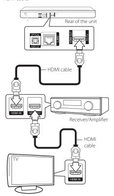
Connect the amplifier's HDMI output jack to HDMI input jack on your TV using a HDMI cable if your amplifier has HDMI output jack. (Refer to amplifier's owner's manual.)
