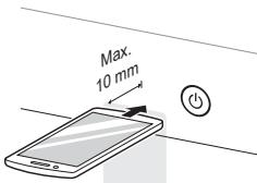
3 Press and hold the **Temp.** button for 3 seconds or longer while holding the smartphone mouthpiece to the **Power** button until the data transfer is complete.
