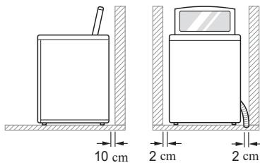
**Level floor:** Allowable slope under the entire appliance is 1°.
