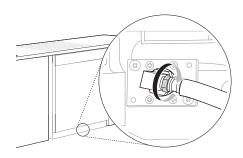
Slide the water supply line back through the channel, pulling gently from inside the cabinet to make sure the line is not kinked, pinched, stressed or crushed.
