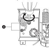
Pair the white, black, and green wires to the matching colored wires from the dishwasher. Then twist on the provided wire nuts **5** tightly to connect the corresponding wires.
