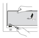
3 Insert a small flat screw driver into the hole of the movable pin. Slide the pin to the right and remove the mini table.
