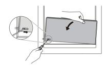
Insert the rubber cover into the hole of the mini table.
