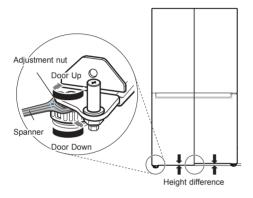
Open the door and use the supplied spanner type 2 to adjust the level of the lower side, using the nut on the adjustable round foot as per the below diagram.
