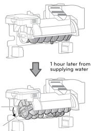
60 minutes after water has been added. to the ice tray, the ice tray will sit slightly tilted to help the cold air reach the ice.
