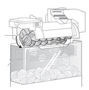
· The ice-detecting sensors will sense when the ice is ready to be dumped into the ice hin
