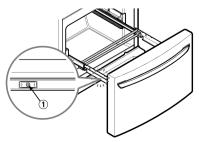
3 Holding both sides of the door pull up to separate the door from the rails.
