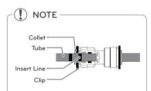
Gently press the Collet and insert the tube until only one line shows on the tube.
