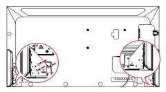
3 Connect the speaker cables noting the correct polarity. Use cable holders and cable ties to organize the speaker cables.
