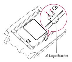
2 After removing the screws, remove the LG Logo. When re-attaching the LG Logo, follow the process in reverse order.
