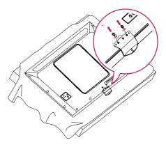
2 After removing the screws, remove the LG Logo. Attach the LG Logo Bracket with the two screws, aligning it with the holes at the right side.
