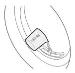
3 Reinsert both inner and outer filter and close the dryer's door.
