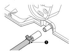
2 Connect the drain hose of the dryer and secure the hose clamp.
