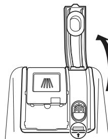
2 Add a liquid rinse aid to the maximum fill level. The rinse aid should be settled in the dispenser while filling, or air bubbles may result in poor drying results.
