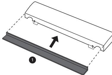
5 Attach the lower cover with the strip onto the appliance.
