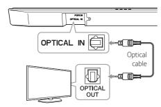
Set up the sound output of TV to listen to the sound through this unit:
