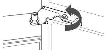
3 Remove the door by raising it from the lower hinge.
