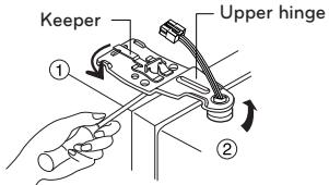
4 Disassemble Door, raising it from Hinge Center.
