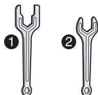
2 (Method 2, only allows a maximum of 3mm of adjustment)
