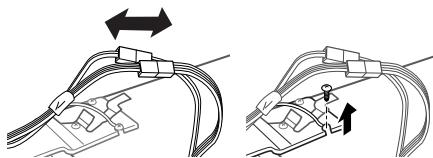
3 Turn ① around to release lock and raise hinge up.
