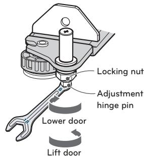
(3) After the door heights are adjusted, completely tighten the locking nut ( ↘ ) counterclockwise.
