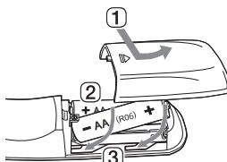
Use AA 1.5V batteries. Replace the two batteries by inserting them into the remote control in accordance with the directions indicated.
