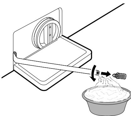
**4** Unscrew the drain pump filter slowly to drain the remaining water and then proceed to remove any debris or objects from the filter.
