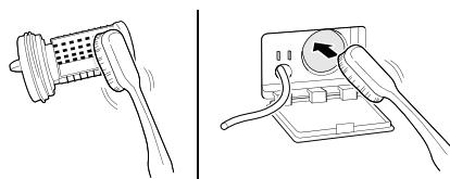
**6** After cleaning the drain pump filter, carefully reinser the filter and screw the drain cap back in clockwise carefully to avoid cross threading and leakage.
