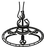
**3** Place the pulsator at its original position and tighten the screw.
