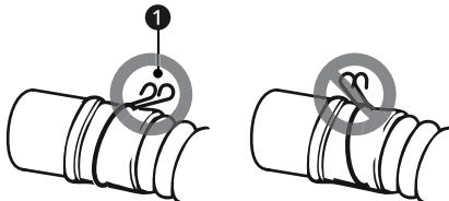
2 Align the drain hose with drain outlet
