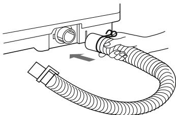
3 Press hose clip and push the hose towards the body of the washing machine and release the snap ring.
