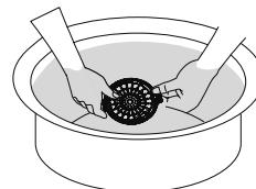
3 Press the upper part of overflow filter down and pull forward.
