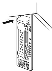
6 Insert the rotation filter-C back into the overflow filter.
