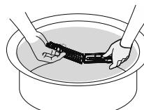
**5** Close the lid and then insert the lower part of the overflow filter into the wash tub and then press top part into original position.
