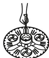
**2** Use a screwdriver to unscrew the screw in the center of the pulsator and lift the pulsator
